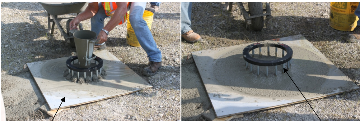
Figure 4-9 The Slump Flow Test With J-ring
