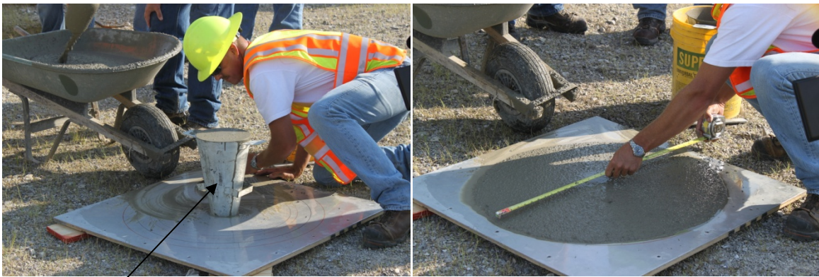
Figure 4-8 The Slump Flow Test Without J-ring
