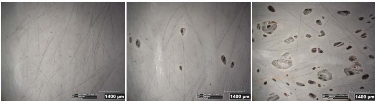
Figure 7-9 Different Percentage of Voids in Control Specimens
