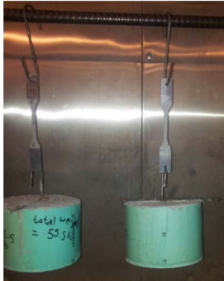
Figure 7-5 FRP Specimens Subjected to Sustained Stress and Thermal Cycles in the Environmental Chamber
