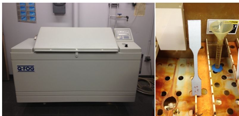
Figure 7-3 Salt Fog Apparatus (Left image) GFRP Specimen Exposed to Salt Fog (Right image)
