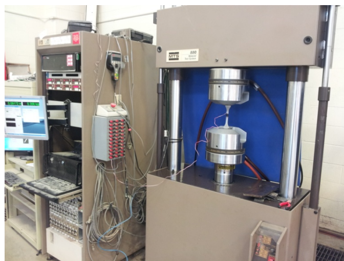
Figure 7-6 Tensile Coupon Test for FRP Specimen via MTS880 Universal Testing Machine
