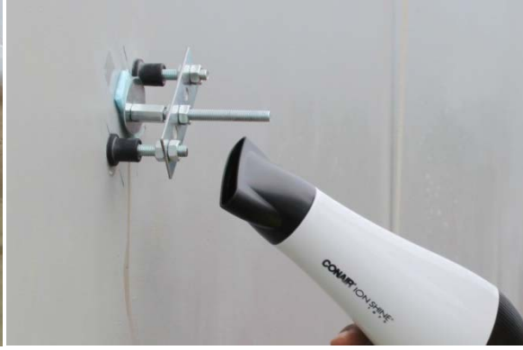
Figure 3-17 FRP Gauge Placement, Constant Pressure for Drying with Added Heat
